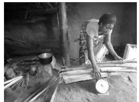
A participant in the stove project weighs the amount of wood she uses for her stove to quantify results.
